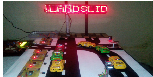
Fig.7. Ultrasonic sensor detected landslide in hilly areas
