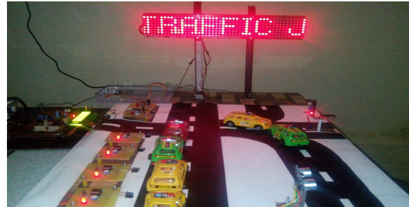
Fig.8. IR sensor detected traffic jam on road
